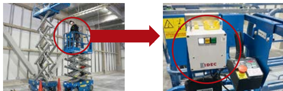
Example installation of the trapping prevention system
